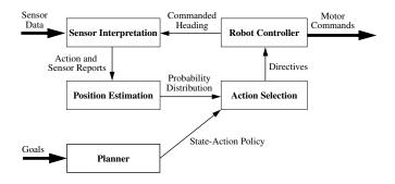
Figure 5: Navigation System Architecture
