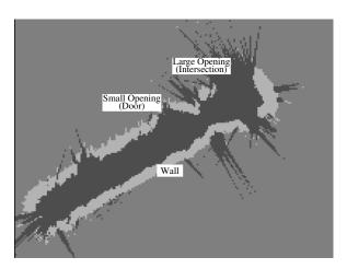
Figure 6: Occupancy Grid with Corridor Features
