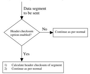
Fig 3. Modifications to the TCP sender
