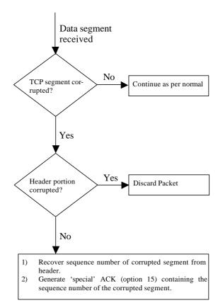
Fig 4. Modifications to the TCP receiver
