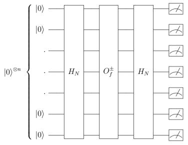
Where  $H_N \equiv H^{\otimes n}$  where  $N = 2^n$ , the  $O_f^{\pm}$  is the  $\pm$  version of the oracle for the function f. After the measurement, if we get  $|0\rangle^n$  we say condition (1) is true, else we say condition (2) is true.
