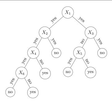
The depth of tree C is 4. The depth of node  $X_1$  is 0 and the depth of  $X_5$  is 2.
