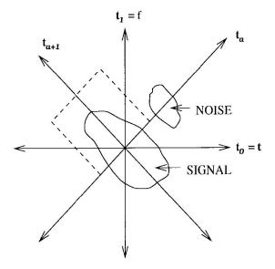
Figure 7: Removing noise from an image with the FrFT.
