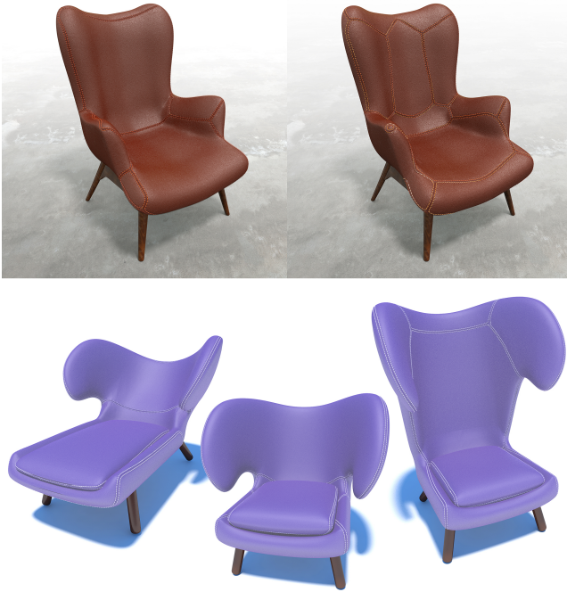
Fig. 2. A variational formulation of cutting makes it easy to explore low-distortion design alternatives. Top : By adjusting parameters in our flow, we obtain designs that look like either classic panelizations for furniture ( top left ) or designs more reminiscent of race car seats ( top right ). Alternatively, we can explore how the changing geometry of a surface affects the cuts needed to easily upholster it ( bottom ).
