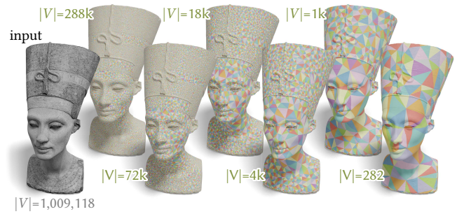
Fig. 29. We can build an intrinsic multigrid mesh hierarchy via repeated coarsening, here reducing the vertex count by a factor 1/4 at each level.
