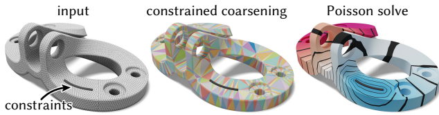
Fig. 28. Fixing vertices during coarsening enables us to exactly preserve boundary conditions and constraint curves when solving PDEs on surfaces.
