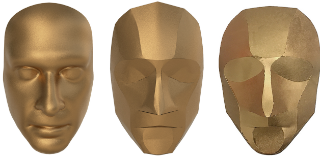
Fig. 24. Simple test of physical feasibility: an initial mesh of a face ( left ) is optimized to obtain a piecewise developable approximation ( center ), which is then cut from paper, glued together, and spray painted to obtain a physical model ( right ).
