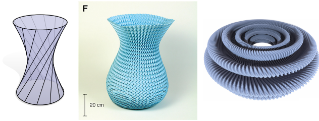
Fig. 6. Merely requiring a surface to have ruling lines does not ensure it can be flattened, such as the hyperboloid of revolution ( left ) which has negative Gaussian curvature. Conversely, a flattenable surface is not automatically ruled unless it is sufficiently regular—consider the C^0 Miura-ori origami pattern ( center ), or the isometric embedding of the flat torus ( right ) which is highly wrinkled even though it exhibits C^1 continuity. We seek a discretization that captures both local flattenability and regularity. (Images from Dudte et al. [2016] and Borrelli et al. [2012], used with permission).
