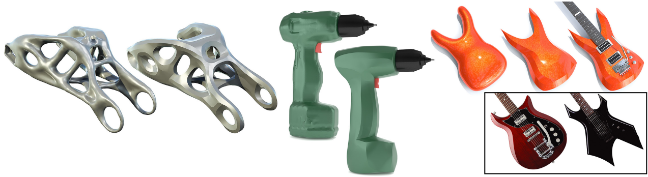
Fig. 21. Here we approximate a given shape (leftmost in each image) with a surface that is developable away from seam curves. Unlike methods that partition the surface into individual pieces, seams can blend organically into the design. Left to right : a swingarm model produced via topological optimization (courtesy Autodesk); the handle of a drill; and a guitar body, which naturally yields features appearing in real guitar designs ( bottom right ).
