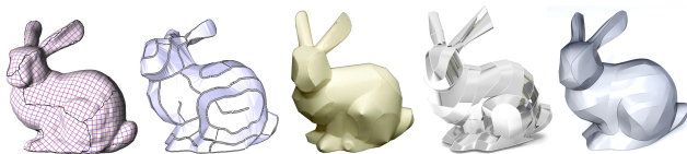
Fig. 3. A variety of methods have been developed to approximate a given surface by easily flattenable pieces. Left to right : Julius et al. [2005], Mitani and Suzuki [2004], Shatz et al. [2006], Tang et al. [2016] (which requires manual editing), and our method.
