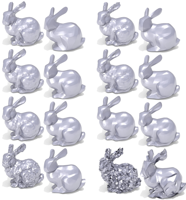
Fig. 27. Different initial meshes lead to different piecewise developable approximations, though the bulk shape typically remains quite close to the input. Overall, fine meshes tend to yield a closer approximation by a larger number of pieces; edges roughly aligned with principal curvatures tend to better preserve geometric features. Moderate noise is typically smoothed out; large amounts of noise can affect the overall shape.
