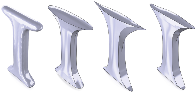
Fig. 10. A given surface ( left ) evolves toward a piecewise developable approximation using the combinatorial energy ( center left ) or the covariance energy ( center right ). Modifying the covariance energy reduces the formation of sharp spikes ( right ).
