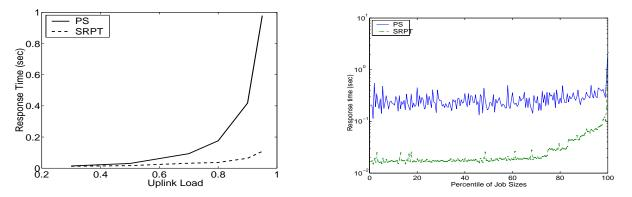
Figure 2: (Left) Mean response time as a function of load for a web server in a LAN environment. Shown under SRPT modification, and under the unmodified, PS, server. (Right) Mean response time as a function of the size of the file requested, for load 0.8.
