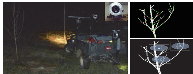
Fig. 1. Mobile robotics system for image-based tree pruning. The system is equipped with a high-resolution flash camera, a Kinect camera and a GPS. Right) In the top the recovered “3D stick” tree representation. In the bottom the suggested pruning.
