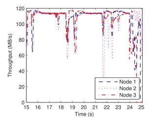
Figure 7: **Aggregate per-node shuffle throughput.** Trace information from the network shuffle microbenchmark is shown for the last 10 seconds of a three-way all-to-all shuffle, smoothed with a 100 ms sliding window. Unexpected network fluctuations and flow unfairness across nodes contribute to partial link utilizations and slower network throughput.
