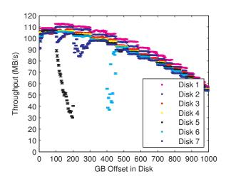
Figure 4: **Full-disk streaming read performance.** Each of the seven representative disks were selected from a set of twenty-five identical-model 1 TB 2009-era disks. Because of new disk manufacturing methods such as adaptive zoning, disk cluster performance has become increasingly variable, creating a heterogeneous environment that complicates efficient job placement strategies.
