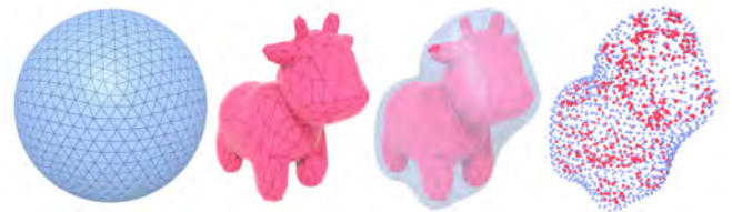
Fig. 27. When using a coarse mesh for our surface ( far left ) and/or obstacles ( center left ) small intersections can occur ( center right ), since our energy discretization approximates each surface by a collection of quadrature points ( far right ). Such artifacts could easily be avoided by, e.g. , checking for collisions during line search.
