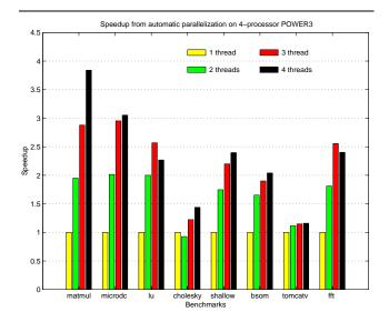
Figure 10: Speedups on a 4-way POWER3 SMP.
