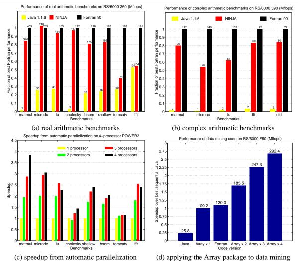
Figure 4: Performance results of applying our Java optimization techniques to various cases.
