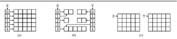
Figure 1: Examples of (a) array of arrays simulating a two-dimensional array, (b) array of arrays in a more irregular structure, and (c) rectangular two-dimensional array.
