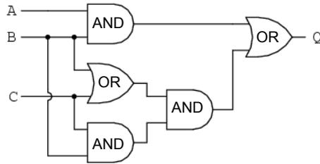
$$Q = (A \wedge B) \vee ((B \vee C) \wedge (C \wedge B))$$
