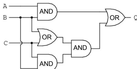
$$Q = (A \wedge B) \vee ((B \vee C) \wedge (C \wedge B))$$
