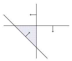
Figure 7.2: The polytope in  $\mathbb{R}^2$  given by the constraints  $-x_1 - x_2 \leq 1$ ,  $x_1 \leq 0$ , and  $x_2 \leq 0$ .
