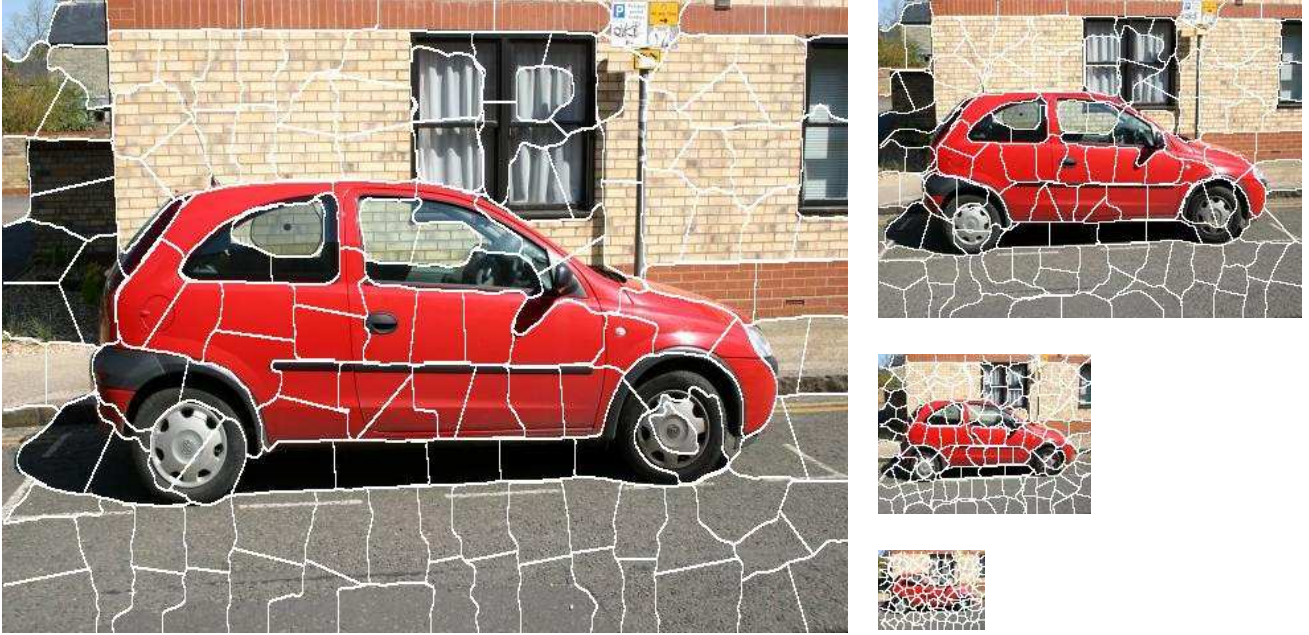
Fig. 5 An example demonstrating that approximately the same number of superpixels (100) can be used at different resolutions with negligible differences in terms of capturing the salient details in the image. Original image (left) is 640 \times 480 pixels. Other images are the result of scaling down by a factor of 2.
