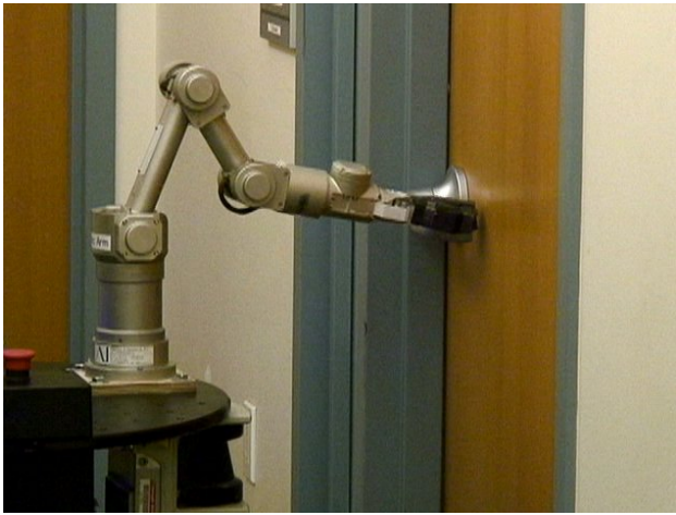
Fig. 8. After localizing the door handle in the 3D point cloud, the robot can plan a path to the handle and open the door.
