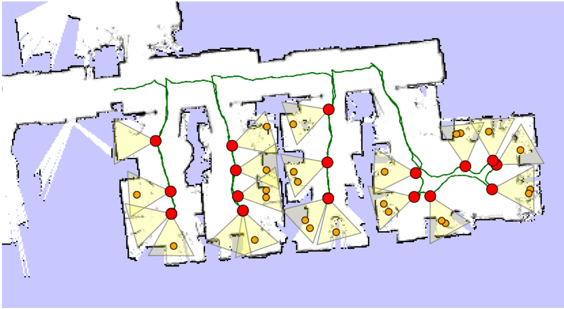
Fig. 10. The inventory-gathering experiment required autonomous navigation (green track), autonomous door opening, and 20 laser scans of desks in the four offices shown above. The robot position at each scan is shown by the red circles, and the field-of-view of each scan is indicated by the yellow triangles. The locations of the detected coffee mugs are indicated by the orange circles. This figure was entirely automatically generated, using the SLAM output for the map and the localization log for the robot track and sensing positions, which allow the coffee-mug detections to be transformed into the global map frame.
