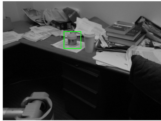
Fig. 9. Detecting coffee mugs in cluttered environments. The detector correctly ignored the paper cup to the right of the coffee mug.
