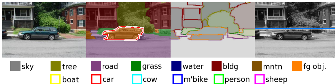
Figure 5.7: Example output from our joint scene decomposition and object detection algorithm. Shown are: (a) the original image, (b) semantic overlay (including object outlines), (c) decomposition by region, and (d) estimated location of horizon.
