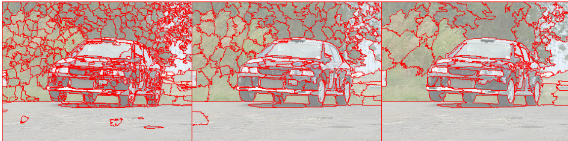
Figure 4.2: Example over-segmentation dictionary, \Omega , for a given image generated by running mean-shift [Comaniciu and Meer, 2002] with three different parameter settings, (h_r, h_s) \in \{(6, 7), (6, 11), (6, 19)\} . The figure shows the boundary of each segment overlaid on top of the original image. In our inference algorithm, each segment \omega \in \Omega defines a set of pixels-to-region association variables \{R_p : p \in \omega\} that may be re-assigned to another region.
