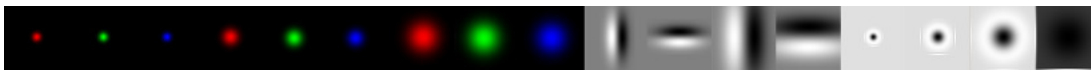
Figure 2.5: Illustration of the 17-dimensional “texton” filters used in multi-class image segmentation [Shotton et al., 2006]. Note that the filters operate in CIELab color space (RGB for the color components shown for illustrative purposes only).
