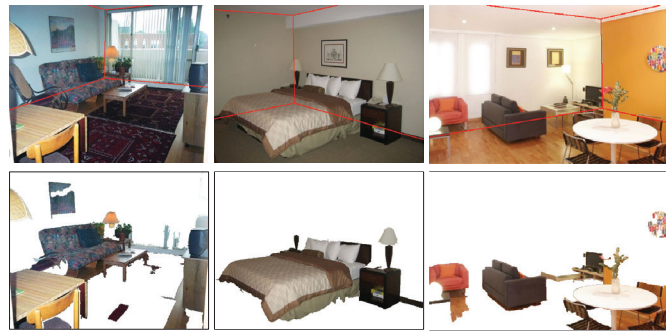
Figure 1. Output of our method. First row: the inferred box layout illustrated by red lines representing face boundaries. Second row: the inferred clutter layout.
