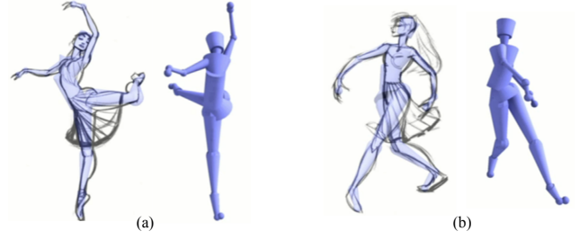
Fig. 7. Collision volumes: The hand-drawings are shown overlaid with the collision volumes. The collision volumes match the drawings approximately, but need not exactly conform to the artist's lines. We also show the collision volumes from an alternate viewpoint.
