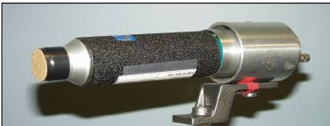
Fig. 9: View of a BGO spectrometer (Harshaw, type NR: 4S4/1.5A – BX) coupled with a photomultiplier tube (Type HAMA 2060)
