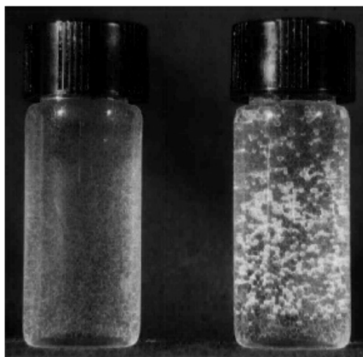
Fig. 3: Superheated emulsions (before and after irradiation)
