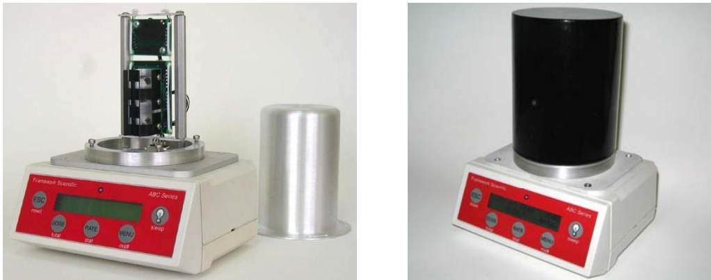
Fig. 4: Photograph of current acoustical bubble counters (open and with lead shell)
