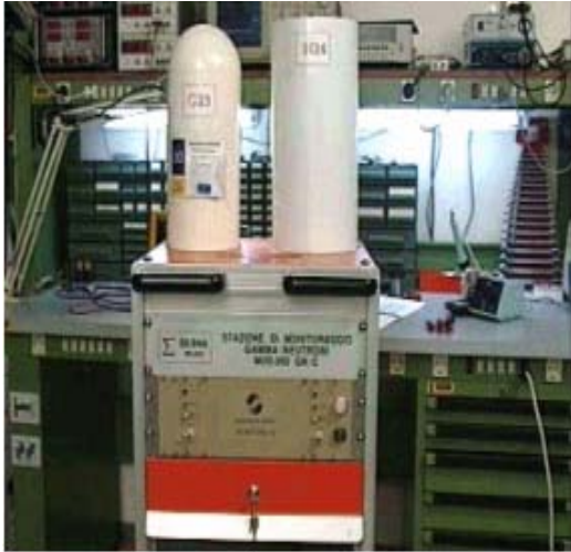
Fig. 18: A gamma/neutron radiation monitoring station at ELETTRA
