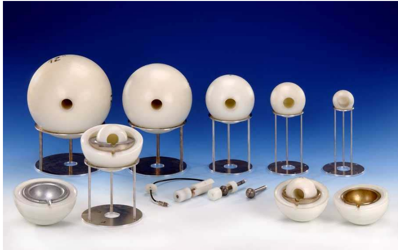
Fig. 1: In the back five of the ten polyethylene spheres ( \text{CH}_2 ) of the PTB NEMUS spectrometer. In the centre, a spherical proportional counter (3.2 cm in diameter) filled with ^3\text{He} gas. In the foreground left and right, parts of the modified spheres. Both the polyethylene and the lead (left) or copper (right) shells are fabricated as half-shells. The combination of spherical shells of different thickness allows different sensitivities to be achieved.
