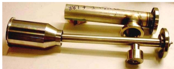
Figure 4: Welding tooling used to minimise deformation.
