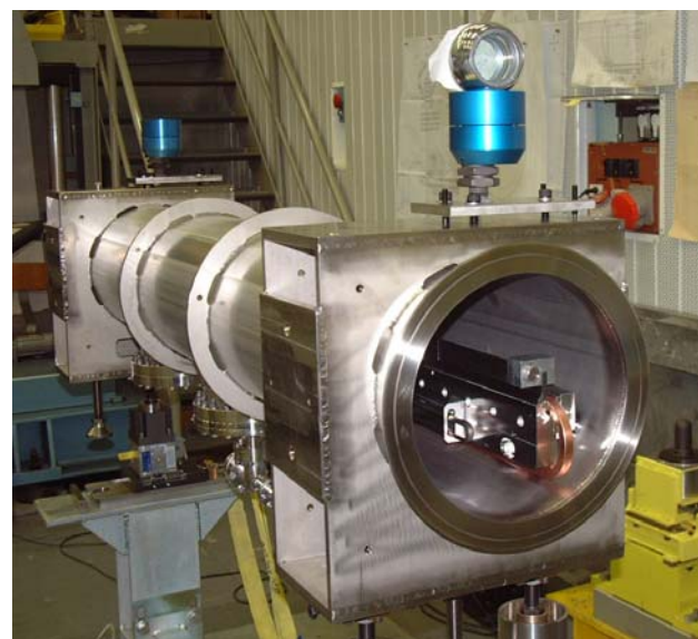
Figure 3: The TPSG6 diluter in its vacuum vessel.
