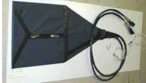
Figure 4. Scintillating tile with two fiber bundles (prototype)
