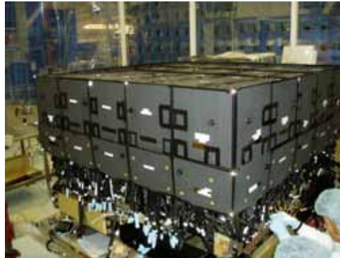
Figure 6. ACD in final phase of integration. Two bottom tile rows are not installed yet (to show fiber cables and PMTs)
