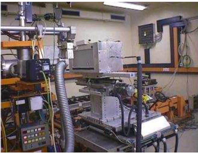
Figure 2: The proton irradiation facility at the compact cyclotron in the Forschungszentrum Karlsruhe. The beam line enters from the left. The beam spot diameter is 1 cm. An insulated box hosts the structures to be irradiated. The box is placed on an x-y stage in front of the beam line, allowing the beam to access a total area of 400 \times 200 \text{ mm}^2 . During irradiation the box is flushed with cold nitrogen gas to prevent annealing due to heating of the structures and to be close to the operating condition at the LHC [5]
