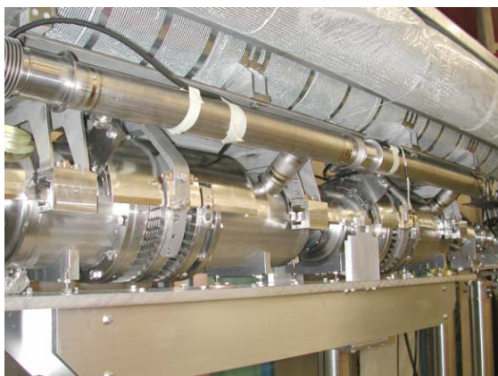
Figure 1: One 2-cavity superstructure, equipped with blade tuners, during assembly in TTF.
