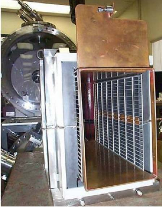
Figure 30: Masking of the ferrite surface of the SNS ring extraction kicker for TiN coating. In order to avoid eddy-current heating, rise-time degradation, and high-voltage shorts, about 20% of the ferrite inner surface is uncoated.
