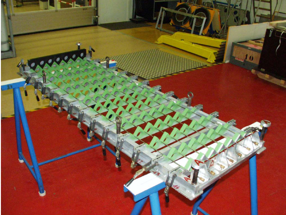
Fig. 16. Tooling used to produce a spacer.
