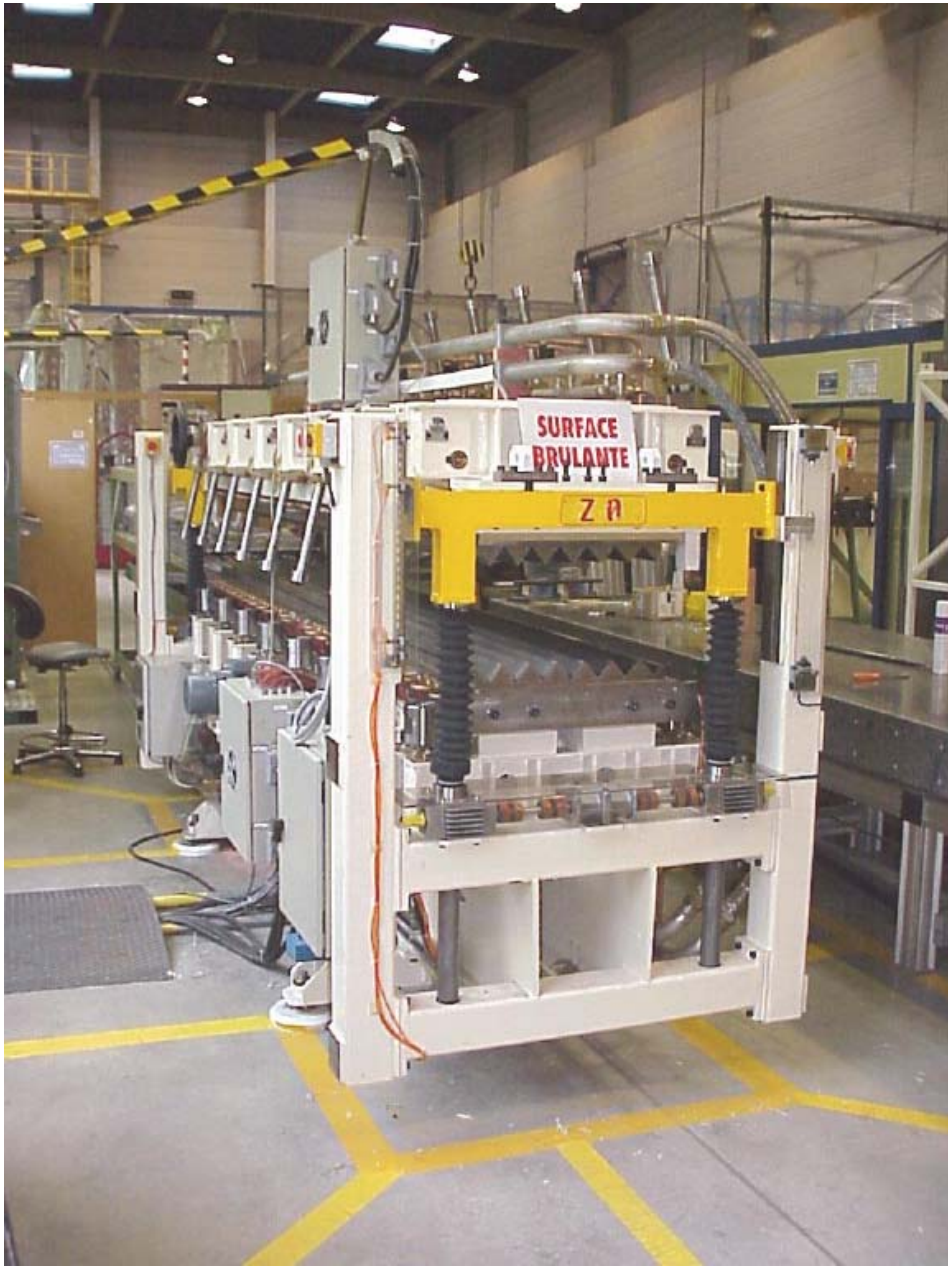
Fig. 11. Picture of the heating press where the absorber is placed for curing after folding.
