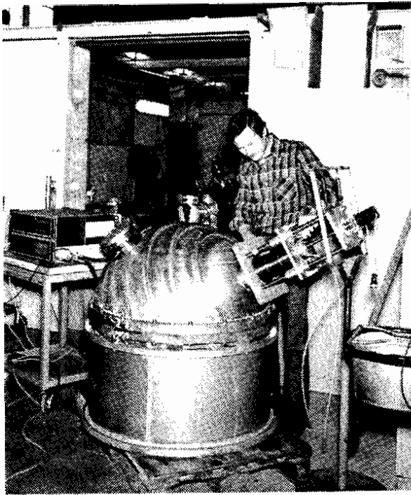
Tetrode the cathode with unmounted grids
