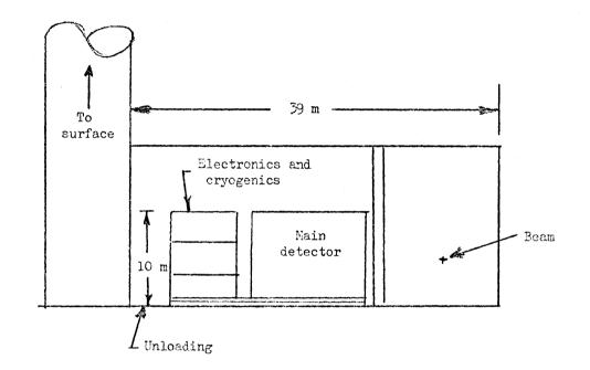
Figure 1 : Hall with one detector in "out" position.
