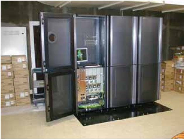
Figure 3: Sony SAIT PetaSite tape library. Seven tape drives, control PC, 16 port fibre channel switch are in the left most console. The left-most console holds 200 tapes (100TB). Each of the right two consoles hold 400 tapes (200TB).
