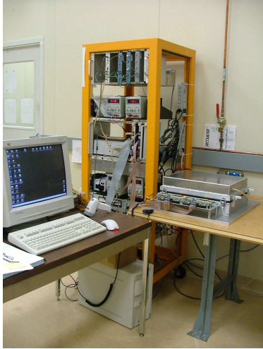
Figure 4: Hybrid thermal test setup.
