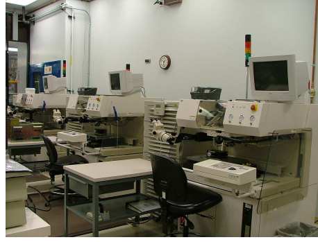
Figure 3: The K & S 8090 wirebonders at FNAL.
