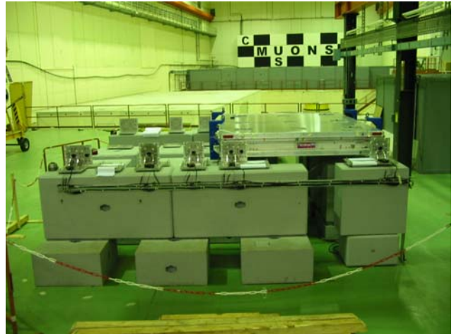
Figure 4: The chamber calibration bench at CERN
