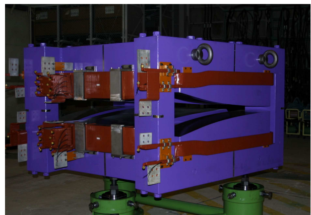
Figure 2: The 150 MeV FFAG DFD triplet. The theoretical field law in the dipoles is of the form B(r) = B_0(r/r_0)^k with B_0 the field at some reference radius r_0 .
