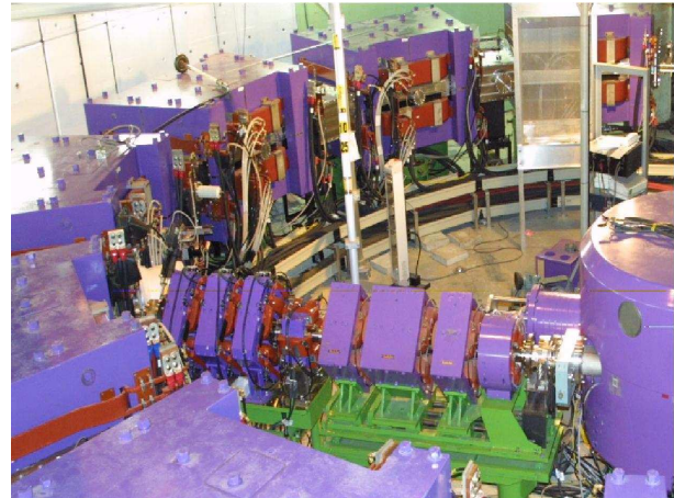
Figure 1: A view of the FFAG ring and of the injection cyclotron and 12 MeV line.
