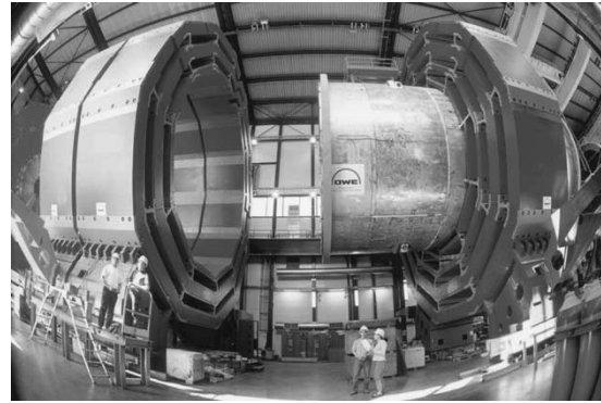
Fig. 1. A recent close-up view of the CMS experiment. The coil, situated inside the external vacuum tank, will surround the calorimeters and tracker. The return yoke, one barrel and two endcaps, comprises three layers of iron in between which will be inserted the muon detectors.
