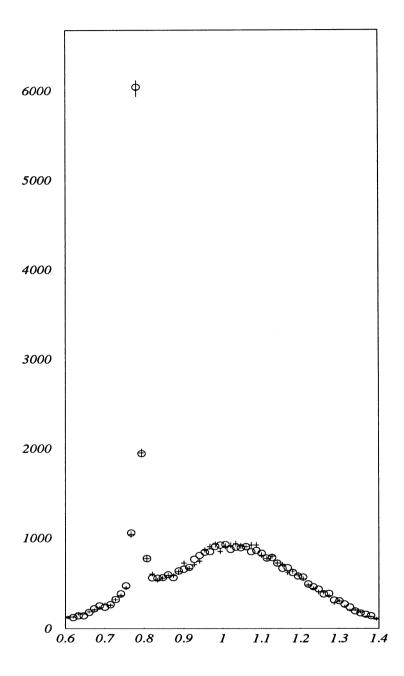
Figure 5: Superposition of the  $\pi^+\pi^-\pi^0$  mass shape with a linear combination of pure  $\rho$  and pure  $\omega$  spectra (circles: linear fit, crosses: full spectrum). The disagreement measures the effect of the interference.
