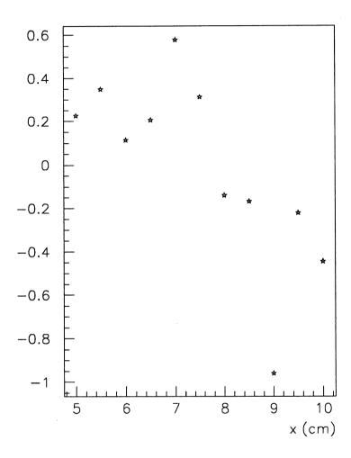
Figure 3: Relative difference in percent between data and Monte-Carlo in the number of events passing the cut on  $x = distance + 2.5 \times energy$  as a function of x
