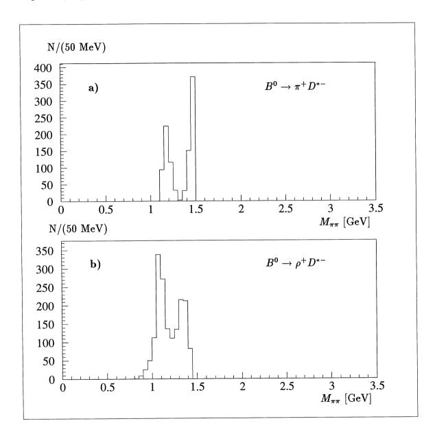
Figure 1.1: Invariant mass of the reconstructed charged pions for a simulation of the decays  $B^0 \to \pi^+ D^{*-}$  and  $B^0 \to \rho^+ D^{*-}$ . Both decays were simulated with longitudinal polarization.
