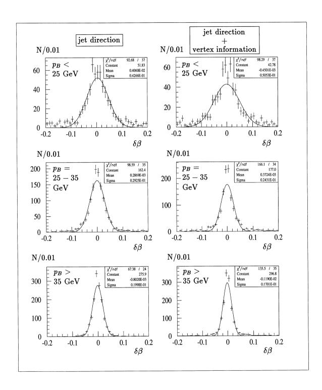
Figure 1.6: Angle between the true  $B^0$  momentum and the reconstruction of the  $B^0$  direction using the jet direction (on the left). On the right sight the vertex information is included.
