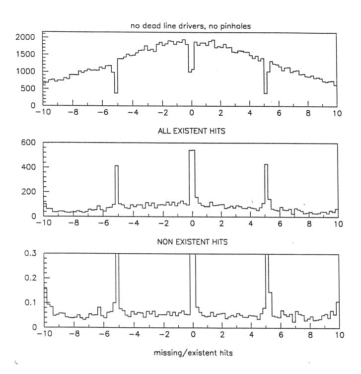
Figure 3: Distribution of the Zcoordinate for sample B (no dead channels). Top: all existing hits, all layers; center: missing hits, the position of the track's impact on the Vdet layer where the hit is missing is plotted; bottom: ratio of top and center plots, bin per bin.
