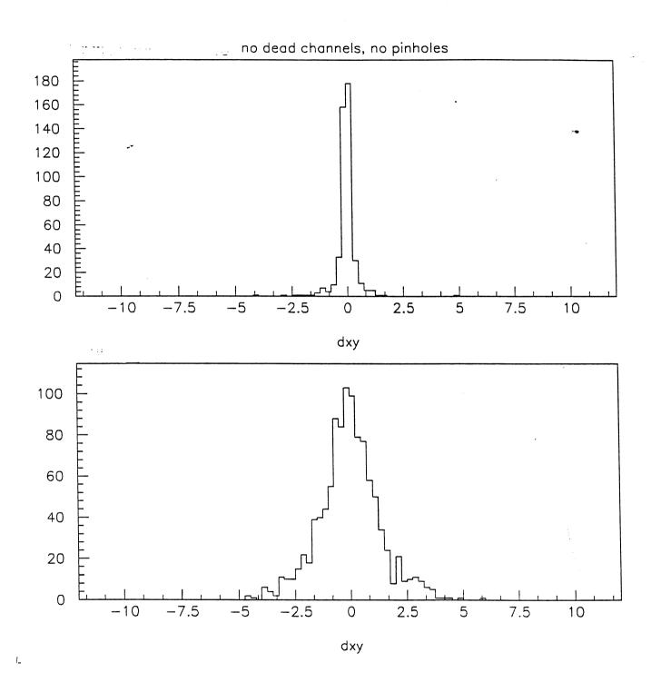
Figure 2: Distance, in the XY plane, between a wrongly associated hit and the impact of the track which caused it. Top: misassociations in the XY view; bottom: misassociations in the Z view.
