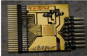
Figure 12: Daughter board with an irradiated APV25 chip.
