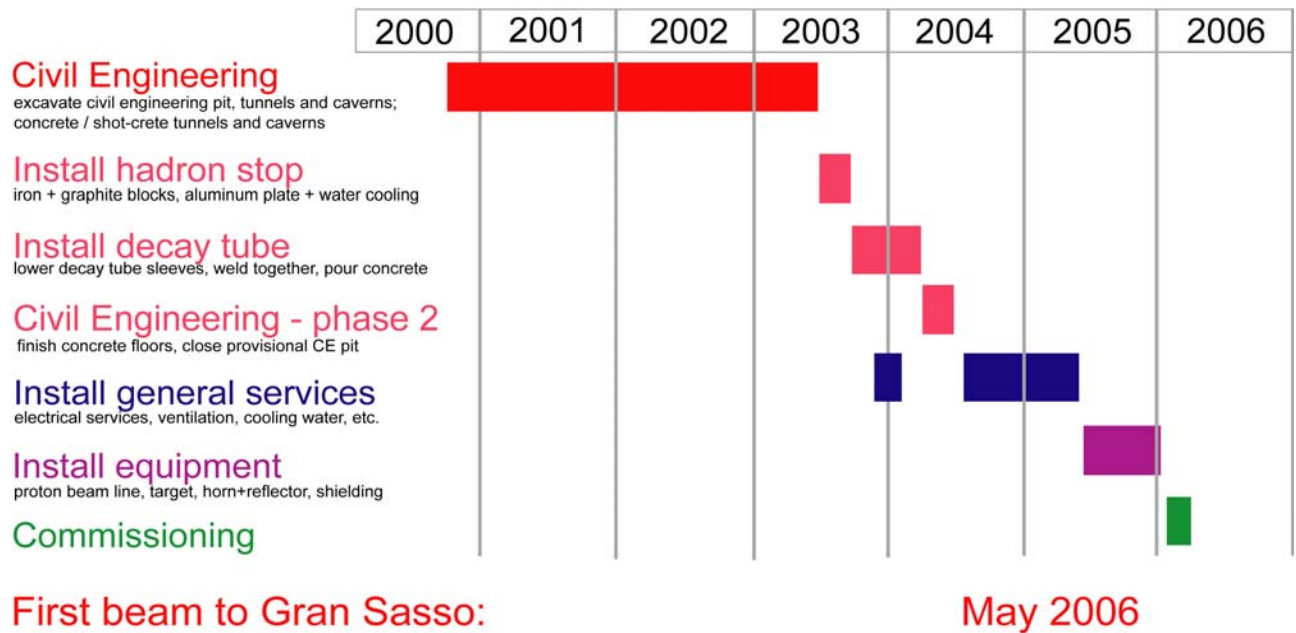
Figure 2.1 - Simplified CNGS construction schedule
