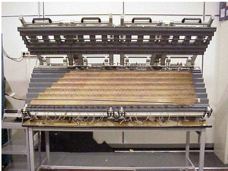
Figure 34: Bench for performing final RC tests on B electrodes
