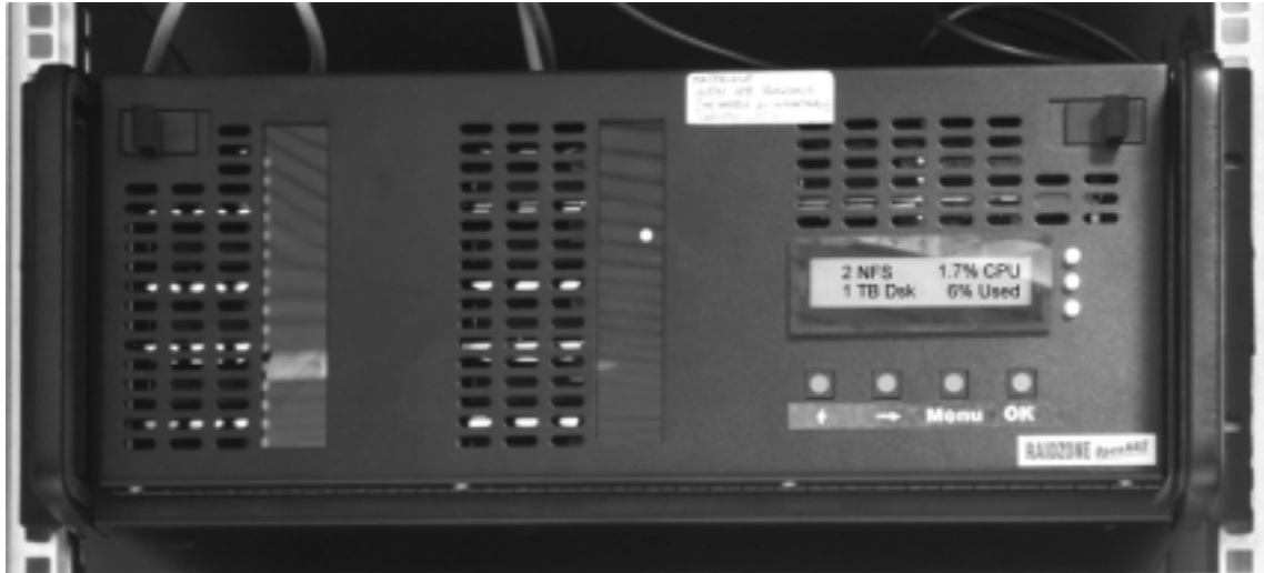
Figure 3: The Network Attached Storage RaidZone RS15-R1200.
