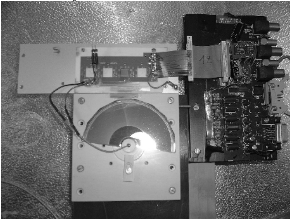
Fig. 4 Rebondable support for the detector. The support can pivot around the centre to allow successive read-out of the various sectors.
