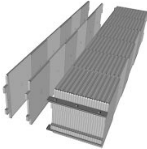
Figure 7: The view of HCAL inner structure. Two master plates shown detached have several spacers glued. The gaps between spacers are used for scintillating tile insertion during optics assembly.
