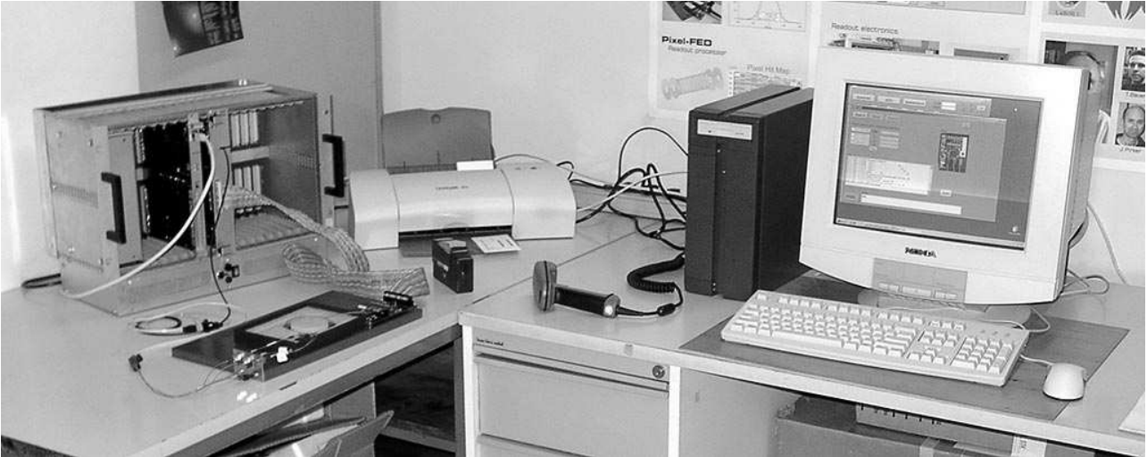
Figure 2. Automatic test setup for the electrical and optical qualification of the AOH.
