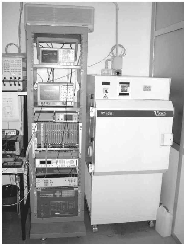
Figure 3. Custom test setup for the electrical qualification of the AOH. On the right is visible the climatic chamber containing the front-end board and the AOH.
