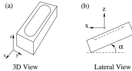
Figure 4: In a tiltmeter: a) Axis definition for the tiltmeter. b) Lateral view for a pure longitudinal tilt.
