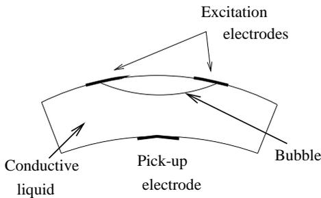
Figure 1: Schematic structure of a tiltmeter.
