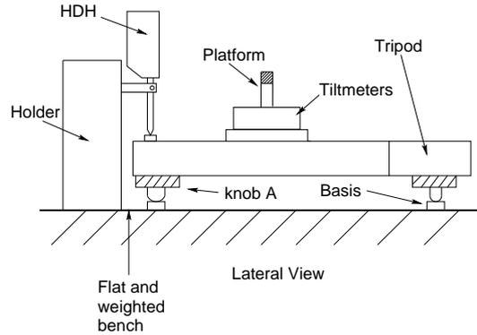
Figure 3: Lateral view of the bench, tripod, tiltmeters and Heidenhain setup. The Heidenhain is supported by a heavy holder, to ensure it does not move when the tripod tilts.
