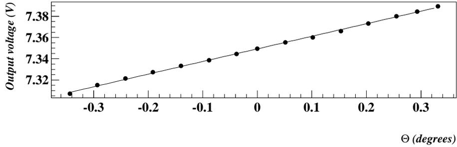
Figure 13: Output response of one of the sensors as a function of the transversal tilt (see text).
