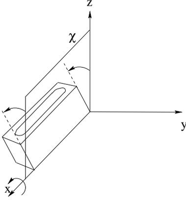
Figure 5: Tiltmeter affected by a transversal tilt.
