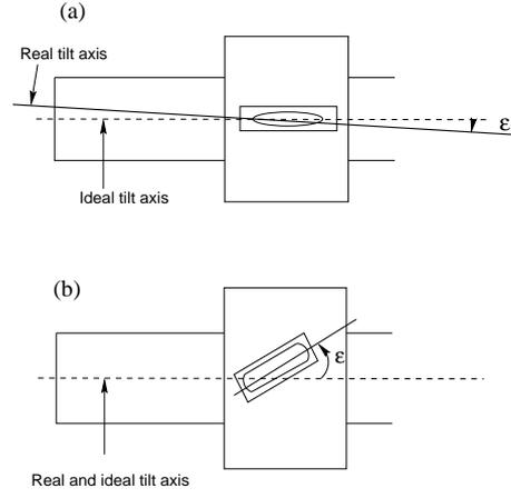
Figure 6: Misalignment angle  $\epsilon$  in a longitudinal tilt. Top view.
