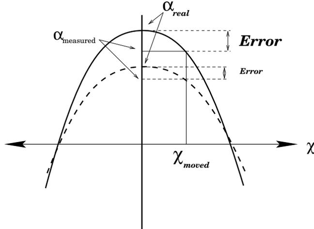
Figure 8: Expected behaviour for the output voltage of the sensors when tilted transversally. The  $\alpha$  angle represents the longitudinal angle measured when the sensor is tilted  $\chi$  transversally.
