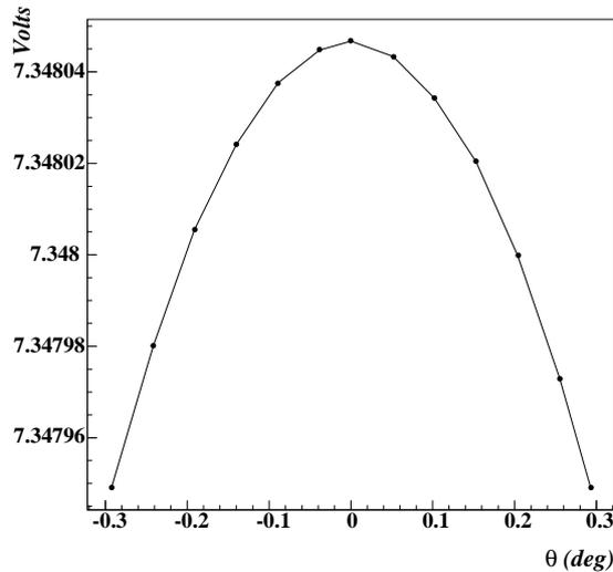
Figure 14: Example of the expected reduction of the output voltage for pure transversal tilts (see text).
