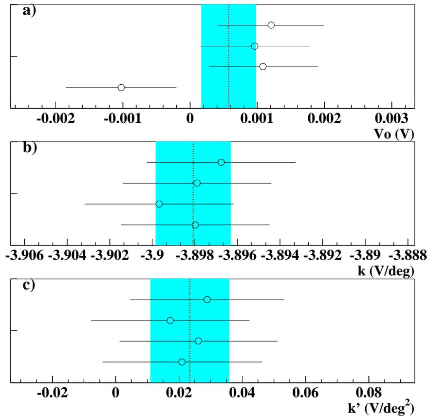
Figure 10: For the four measurements carried out (see text): a) tiltmeter offset, b) linear factor and c) quadratic term. The global average is the dotted line and the shaded area is the global rms.
