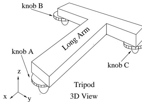
Figure 2: 3D view of the tripod used in the tests.
