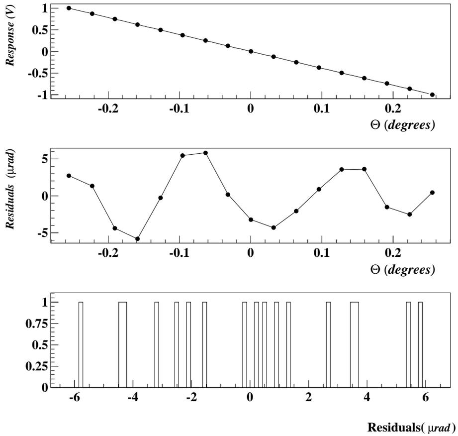
Figure 9: From a longitudinal calibration: a) Output voltage as a function of the tilt fitted to a quadratic polynomial. b) The residuals from the fit as a function of the tilt. c) The distribution of the residuals.
