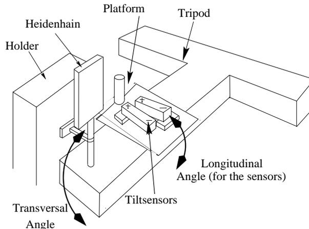
Figure 12: 3D view of the arrangement of the sensors during a transversal calibration. The sensors are lifted using wedges.
