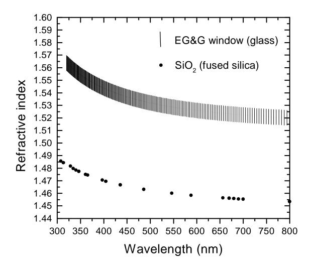
**Fig. 3:** experimentally determined refractive index of the EG&G APD window compared with the one of the SiO<sub>2</sub> (fused silica) [5] which, as discussed in the text, is assigned to the EG&G transparent glue (TG). In the same wavelength range, the extinction coefficient of the glass window is  $k < 1 \cdot 10^{-6}$ .
