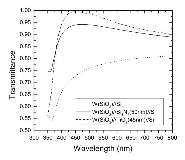
**Fig. 8a:** transmittance from  $W(SiO_2)$  to the Si without and with  $Si_3N_4$  (50nm) and  $TiO_2$  (45nm) AR.
