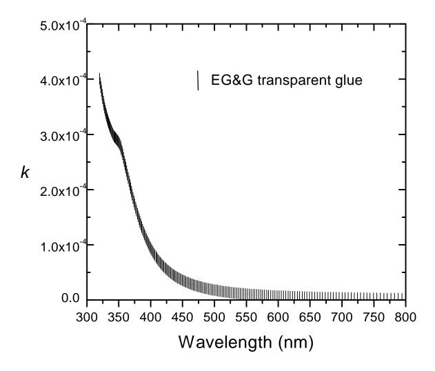
**Fig 5b:** extinction coefficient of the 30µm thick transparent glue (TG) layer, placed between window and Si in the EG&G APD, giving a good reproduction of the experimental reflectance measurement.
