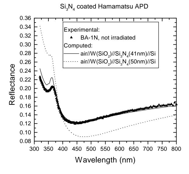
**Fig. 7:** reflectance of the  $Si_3N_4$  coated "BA1N" Hamamatsu APD compared with the computed reflectance based on the model "air//W( $SiO_2$ )// $Si_3N_4$ (41nm)//Si". The effect of the  $Si_3N_4$  antireflection coating is more effective in the 400-520 nm range when the coating thickness is about 50 nm.
