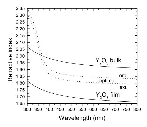
**Fig. 10:** refractive indexes of: a) the optimal AR coating for the PWO//DG interface  $(\sqrt{n_{PWO}n_{DG}})$ , both for the ordinary and the extraordinary PWO refractive indexes; b) Y<sub>2</sub>O<sub>3</sub> bulk [7]; c) Y<sub>2</sub>O<sub>3</sub> film deposited on the PWO test piece as computed from the measurements reported in Fig. 11.
