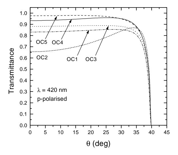
**Fig. 14b:** computed *p*-polarised transmittance, from the PWO to the Si, versus the incidence angle at 420nm for:
