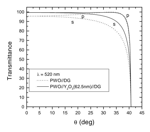
**Fig. 13b:** simulated transmittance versus incidence angle at 520nm of the interfaces PWO//DG and PWO// $Y_2O_3(62.5nm)$ //DG.
