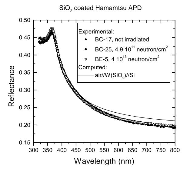
**Fig. 6:** reflectance of BC-17, BC-25 and BE-5 Hamamatsu APD, irradiated with neutrons at several doses compared with the reflectance computed according to the model "air//W//Si", where the refractive index of the rubber window (W) is assumed to be the same of the SiO<sub>2</sub> coating.
