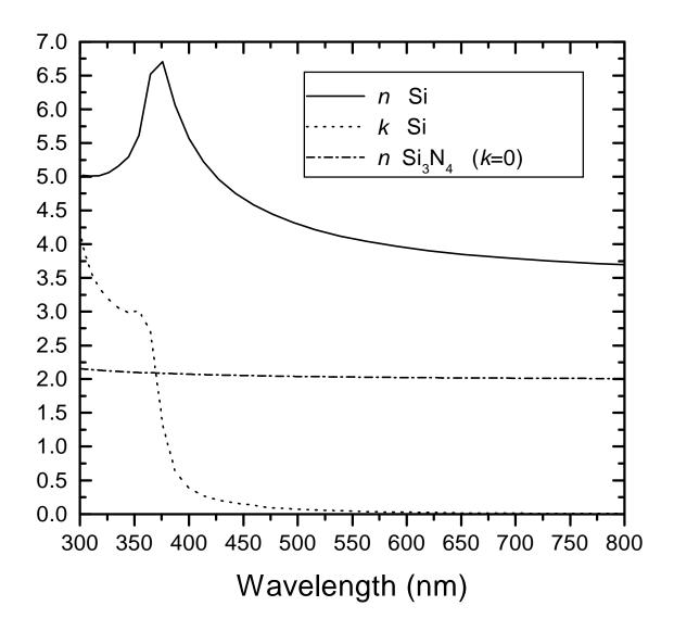
Fig. 5a: complex refractive indexes of Si and Si<sub>3</sub>N<sub>4</sub> [5].
