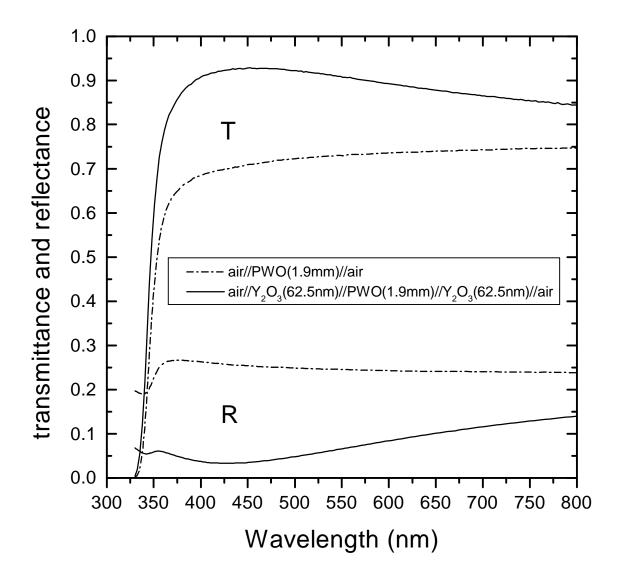
**Fig. 11:** transmittance and reflectance, at normal incidence, of the uncoated and coated PWO test piece. The experimental curves are well reproduced by assuming the films perfectly transparent (k=0), 62.5 nm thick and with the refractive index of a material composed by 76% in volume of  $Y_2O_3$  [7] and 24% of air, computed according to the effective medium approximation [9].
