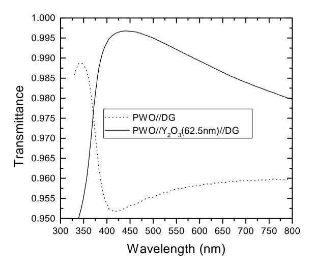
**Fig. 12:** simulated transmittance, at normal incidence, of the interfaces PWO//DG and PWO// $Y_2O_3(62.5nm)$ //DG. With the AR coating the transmittance is about 4% greater than the uncoated case.
