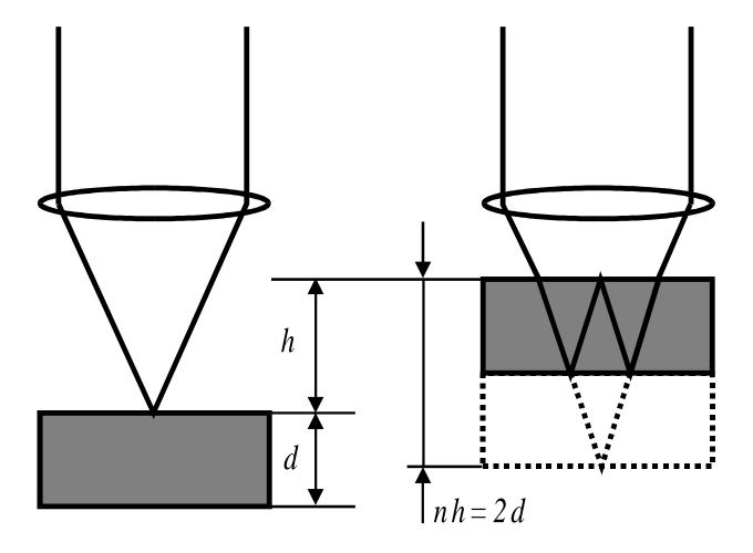
**Fig. 2:** determination of the window thickness (d) by an optical microscope: the difference between the heights of the microscope plate (h) for which, respectively, the window external surface and its image (reflected by the Si surface) are focused, correspond to the optical path nh = 2d, where n is the refractive index of the window.
