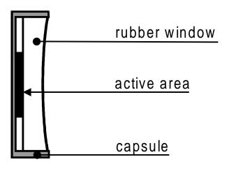
**Fig. 1:** section of APD's produced by EG&G and Hamamatsu. In both devices the Si wafer is enclosed in a capsule and covered with a transparent window. In the EG&G APD (Fig. 1a) the window is sealed to the capsule with some transparent glue. The Hamamatsu (Fig.1b) adopts a rubber window which completely fills the capsule-room and cover the Si surface together with the electric contacts (not reported in the figure).
