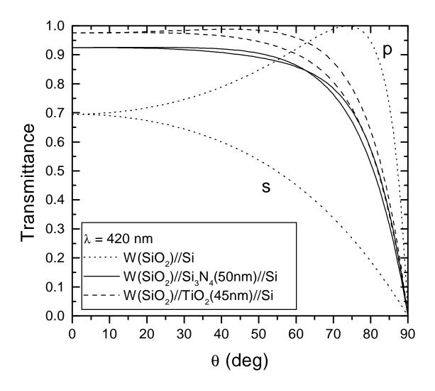
**Fig. 8b:** transmittance at 420 nm versus the incidence angle from  $W(SiO_2)$  to the Si without and with  $Si_3N_4$  (50nm) and  $TiO_2$  (45nm) AR.
