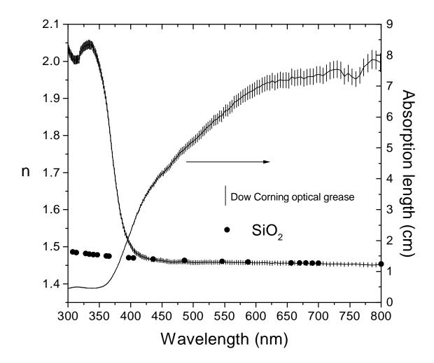
**Fig. 9:** measured refractive index and absorption length of the Dow Corning 02-3067 optical grease. For wavelengths greater than 400nm the refractive index is very similar to the  $SiO_2$  (fused silica) one, also reported in figure [5].
