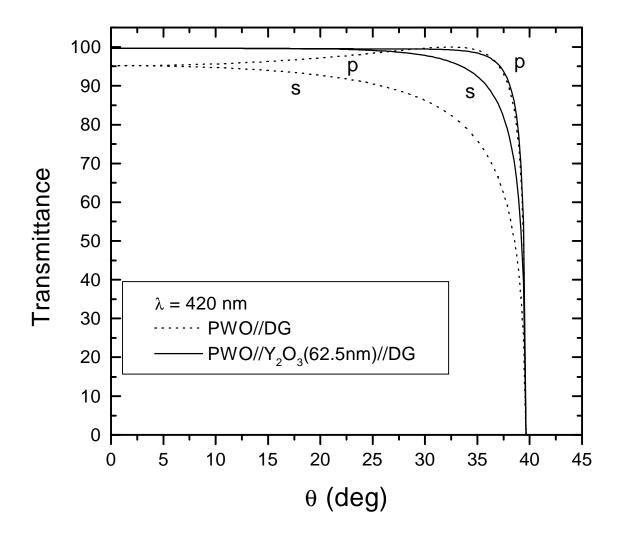
**Fig. 13a:** simulated transmittance versus the incidence angle at 420nm of the interfaces PWO//DG and PWO// $Y_2O_3(62.5nm)$ //DG.
