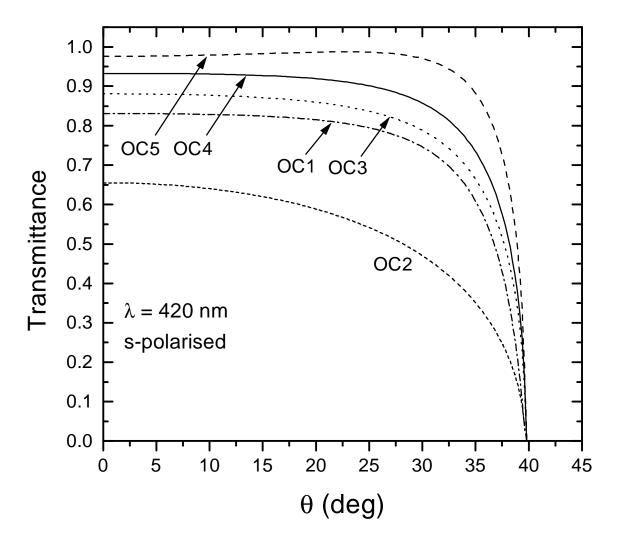
**Fig. 14c:** computed *s*-polarised transmittance, from the PWO to the Si, versus the incidence angle at 420nm for:
