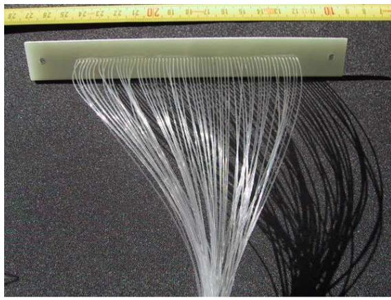
Figure 6: Mechanical structure of the fibre array that is mounted on the test box. The size of one LED spot is equivalent to approximately 30 detector strips when the array is fixed 3 mm above a silicon wafer.
