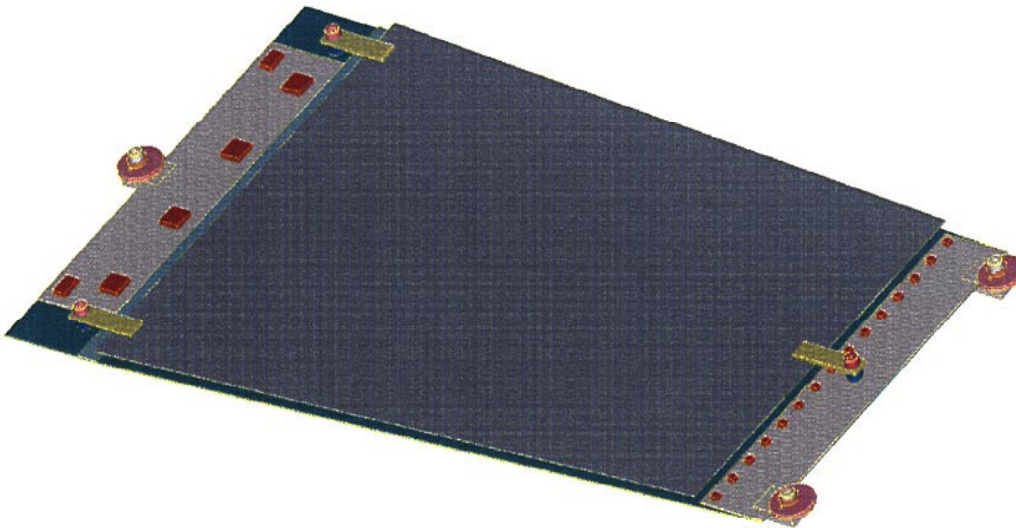
Figure 18 : Assembly of an individual forward MSGC.
