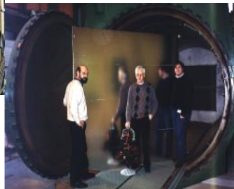
Figure 10 : Composite panel at the exit of the autoclave at the SABENA plant.
